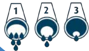
b) Grease Clogging in Pipes
